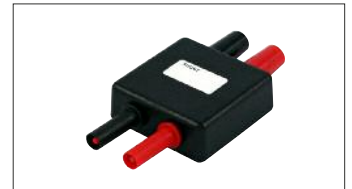
912008000: 10 ohms shunt, 0.1%, 0.15A max
